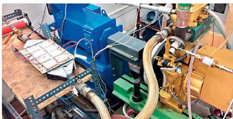
View of the hydrogen-fuelled engine set-up for testing the energy harvesting silencer.
